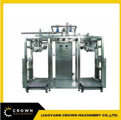
The purpose of this filler is to pack the sterilized coconut milk in a sterile environment so as to obtain a longer shelf life without preservatives and without refrigeration.
