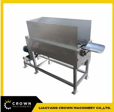
This machine serves the purpose of removing the old coconut husk ( coir) with the fine knife teeth install on two rotational screw rollers, the husk discharge from a slide way at bottom.
